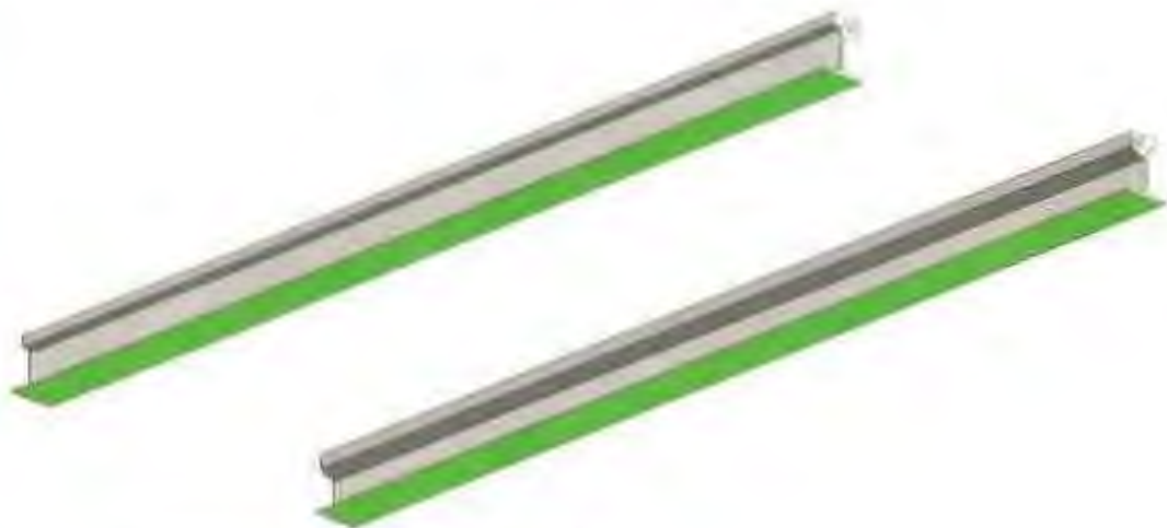
Picture: continuously supported rail
