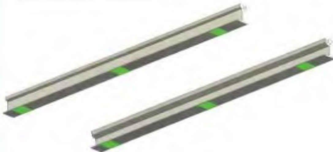
Picture: discrete supporting points (green marks)
