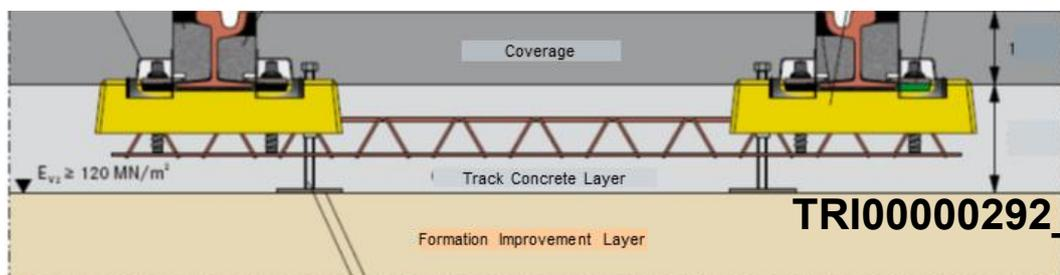
This required beneath it a formation or track improvement layer consisting of a reinforced concrete slab capable of achieving 120MPa support for the life of the trackform [TRI00000183\_0003, paragraph 3.1 and **Public Hearing Transcript, 5 December 2017, page 30:13-22**]. By way of illustration, reference is made to the diagram on page 7 of Mr Foerder's Supplementary Witness Statement [TRI00000183\_0007], an extract of which is copied below:
